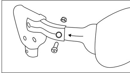
Secure the backstrap into position by inserting the screw and nut. The nut should be positioned into the hexagon shape hole on the inside of the backrest connector. Tighten securely using a Phillips screwdriver.
