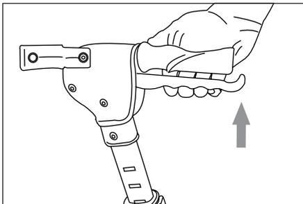
Push down on brake handle to lock the brake into PARK.
