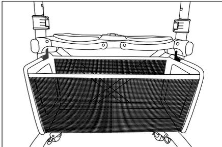
Loop the strap (velcro) around the frame and insert into wire tab.
