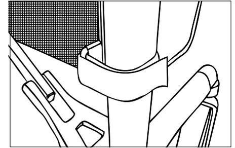
Insert red clip into basket hook. Red clip will 'click' when locked into position
