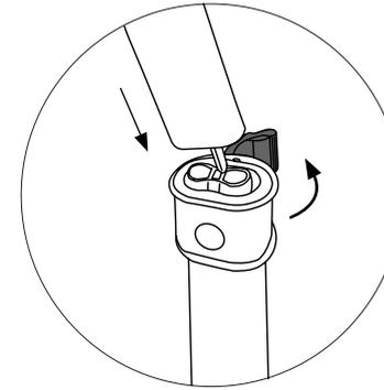
While holding the GREY release lever in the open position, slide the brake handle into the frame.
