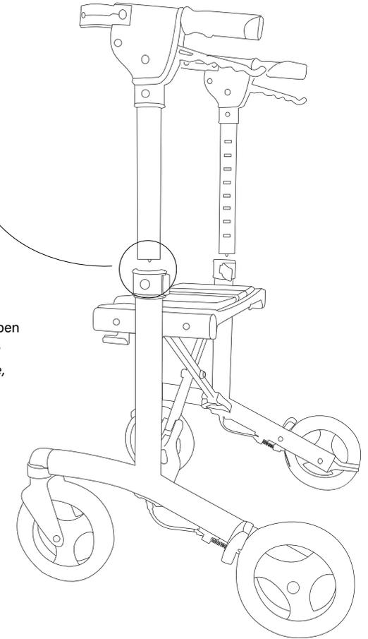
The metal rod protruding from bottom of brake handle tube must be inserted into the rectangular slot in the middle of the frame. Set the desired handle height (The line below the number on the handle should line up with the top edge of the frame), and close the GREY lever. The release lever should 'click' when locked into the closed position.
